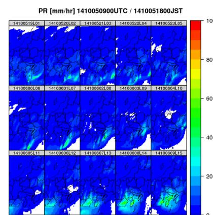
Ground radar-observed rainfall data with spatiotemporal resolution 1km and 5 min (upper)
