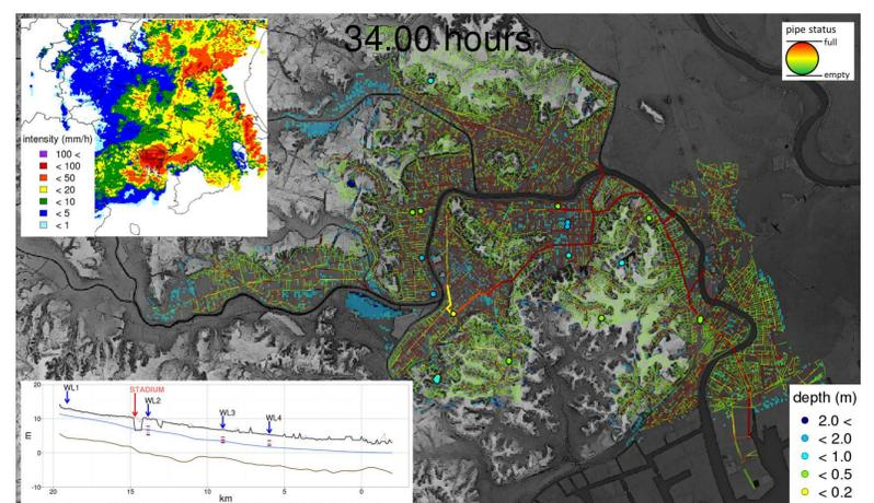
Simulated urban inundation by the data-archive integrated model at the typhoon Phanfone 2014. The map shows drainage network status of flow capacity where darker red colors indicate full capacity and dots indicate drained water may flow out through manholes. It also shows the ground radar-observed rainfall data (upper left) and river water level (lower left). Visualization is done in R environment with fields, ggplot2, grid, raster, rgdal, rgeos, libraries
