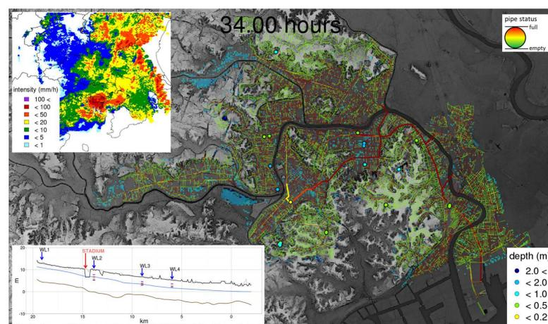
Simulated urban inundation by the data-archive integrated model at the typhoon Phanfone 2014. The map shows drainage network status of flow capacity where darker red colors indicate full capacity and dots indicate drained water may flow out through manholes. It also shows the ground radar-observed rainfall data (upper left) and river water level (lower left). Visualization is done in R environment with fields, ggplot2, grid, raster, rgdal, rgeos, libraries
