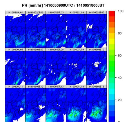
Ground radar-observed rainfall data with spatiotemporal resolution 1km and 5 min (upper)
